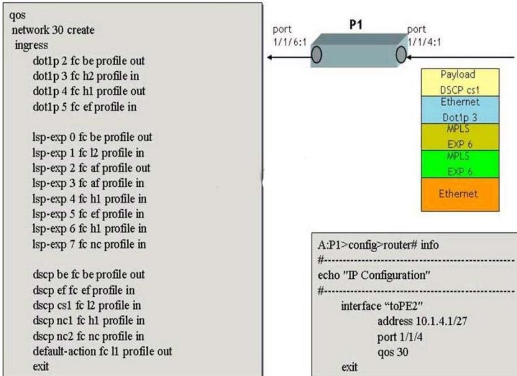
Based on the configuration of the network policy (below), what will be the forwarding class associated with a MPLS encapsulated customer packet that arrives on a dot1Q encapsulated network port 1/1/4:1 on P1 with the following characteristics:
